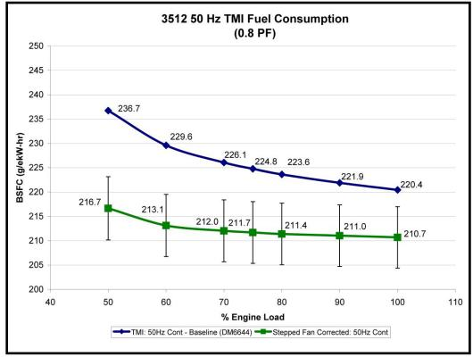
Stepped Fan Corrected data shows 3% error bars at each data point
