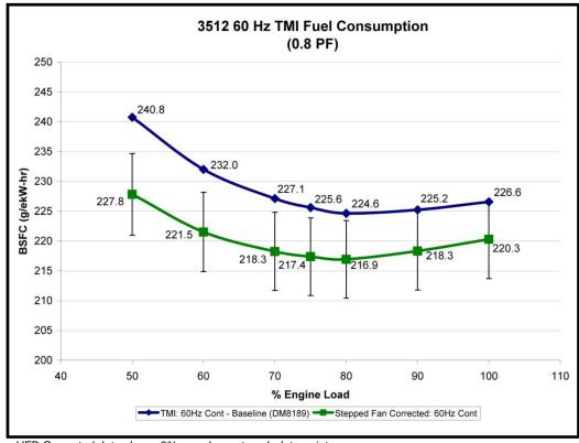
VFD Corrected data shows 3% error bars at each data point
